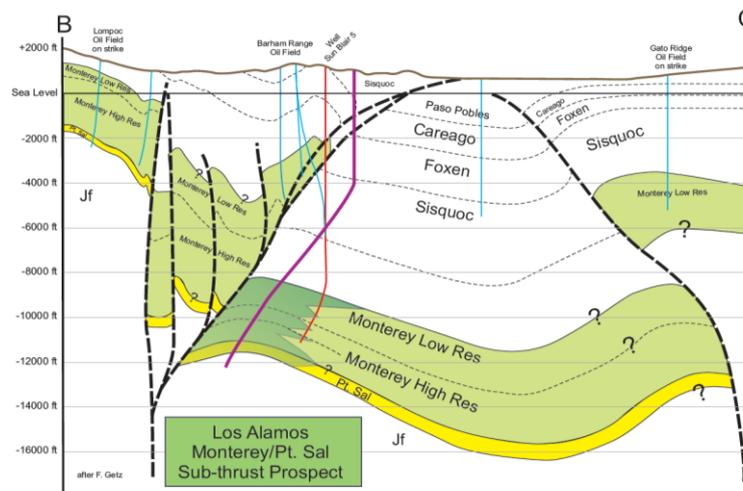
Cross section of the large target Monterey shale
